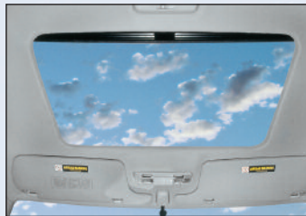
Sunroof panel vents or opens fully.
