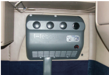
The in-cab mounted air handler delivers chilled air to the bunk for up to 10 hours without consuming any fuel at discharge.
