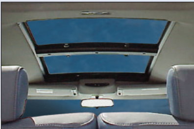
Interior, all 4 sunshades open.
