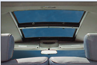
Interior, all 4 sunshades open.
