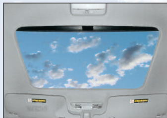
Sunroof panel vents or opens fully.
